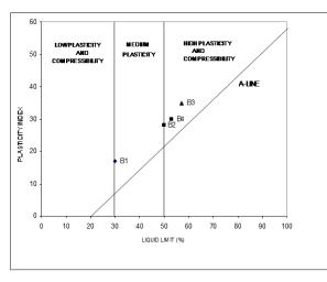
Fig. 3. Casagrande chart classification of soils from pit B
