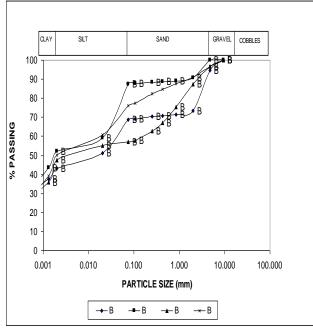
Fig. 5. Grading curves of soils from pit B
