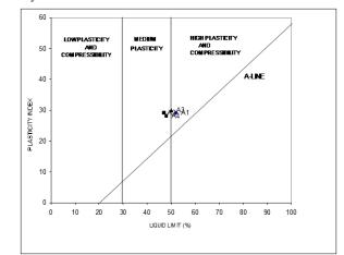
Fig. 2. Casagrande chart classification of soils from pit A
